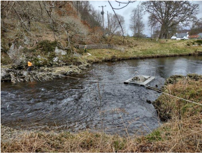
Photo 3: Farrar downstream box trap (KOS), NH35556 39332 With extra guide rope on surface.
