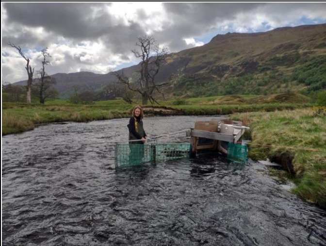
Photo 5: Farrar West Arm box trap (Strathconon), NH 26484 38037. Double wing intercepting flow.
